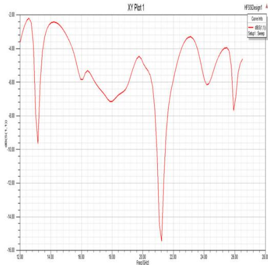
**S-Parameter Result for Reconfigurable Antenna**
